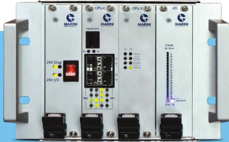
The main purpose of the Safe Data Transmission System (TDS) is to replace the copper cables which is the most common means used for safety link in railway signalling systems. The TDS system is composed by a set of U-TDS devices. The devices communicate each other by using the PVS safe protocol through an LAN network.
