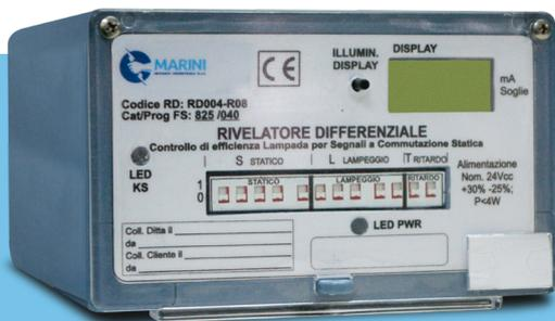
The Differential Detector (RD) measures the True RMS current absorbed by the lamp of the Colour Light Signals Italian SDO type and excites an external relay called KS (typical Italian FS 58 type), only if the measured RMS current value is within the preset range. The RD is approved according to the RFI DTCDNSSSTB SF IS 05 760 B Italian Railway Specification.
