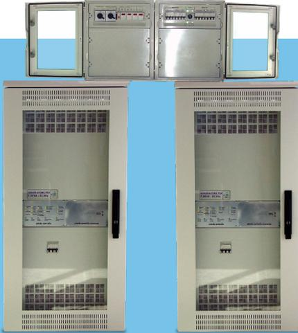
The PSK 83.3Hz Generator was engineered and produced in collaboration with Tekfer Industries. It can supply track circuits with 83.3Hz alternating voltage and modulated with the specific phase modulation law (PSK). Two regulated voltages Indoor (Locale) and Outdoor (Campagna) are generated; its value can be set to a predetermined range by means of a dedicated connector block.
