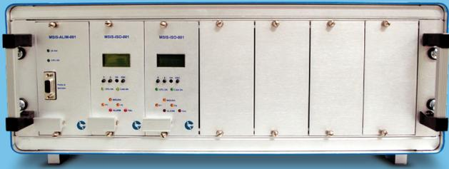
The MSIS system measures the insulation of a Signalling System (IS) cable to Earth or to Equipotential Bar of the power supply system. The system is able to detect insulation anomalies.
